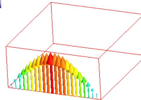
*This rectangular waveguide contains a symmetric propagating mode, which could be modeled using half the volume vertically....*
